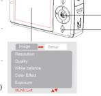
Press OK/Enter on the five-way control button (1) to save the settings and finally press the MENU button (2) to close the menu
